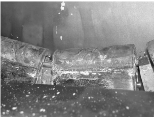
Fig. 4. View of LLL surface after series of discharges with additional plasma heating.
